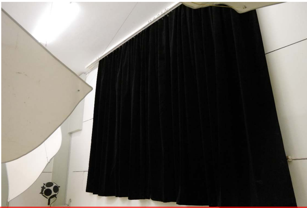
Figure B.1. Fabric in the reverberation room, flat arrangement.
