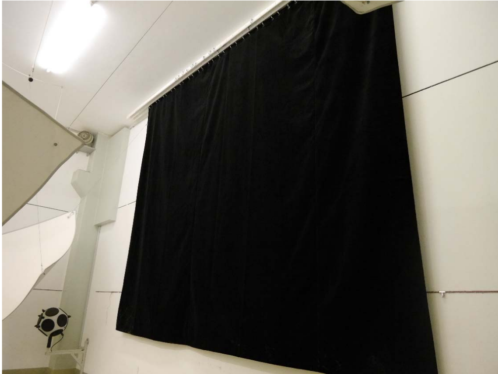
Figure B.1. Fabric in the reverberation room, flat arrangement.
