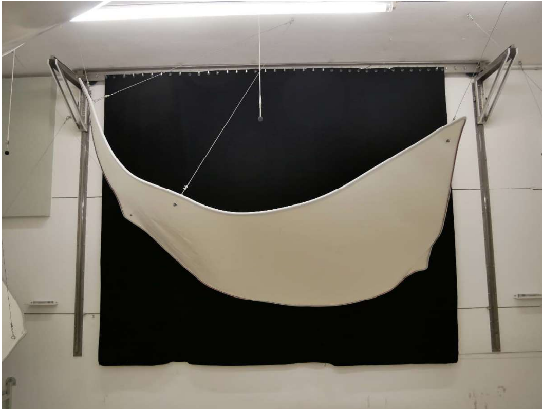
Figure B.1. Flat test arrangement in the reverberation room (frontal view).
