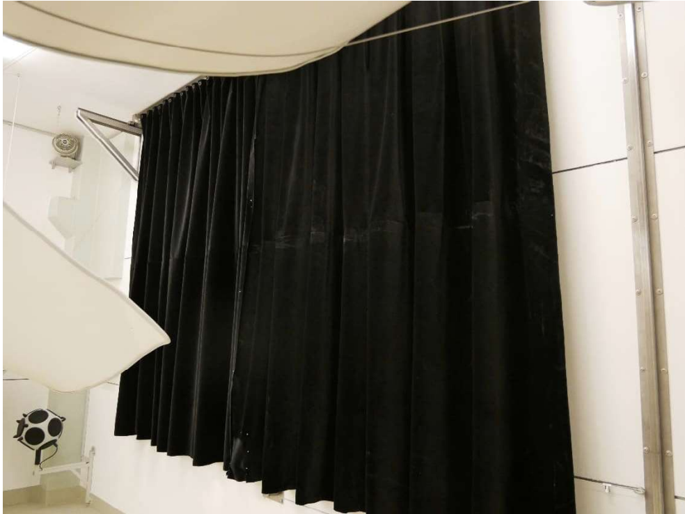
Figure B.3. Pleated hanging curtain, 100 % fullness in the reverberation room: diagonal view.
